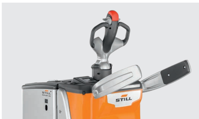
Safe support on both sides for operators thanks to the side bars
