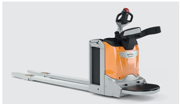
For even more productivity in horizontal goods transport, the EXH-SF 16C/20C is optionally available with 2,400 mm forks
